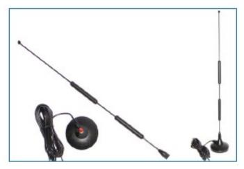
**Technical Data:** Frequency: 700-900 MHz / 1800-2100 MHz / 2400-2700 MHz Impendance: 50 Ohm V.S.W.R.: 2.0:1 Gain: 5 dBi Polarization: vertical Max. Power: 10W Temperature range: -40°C to +80°C Cable: RG58 - 3,5 m Connector: SMA (male) Base: magentic, 70mm Ø Hight: 453mm Weight: 249 g
