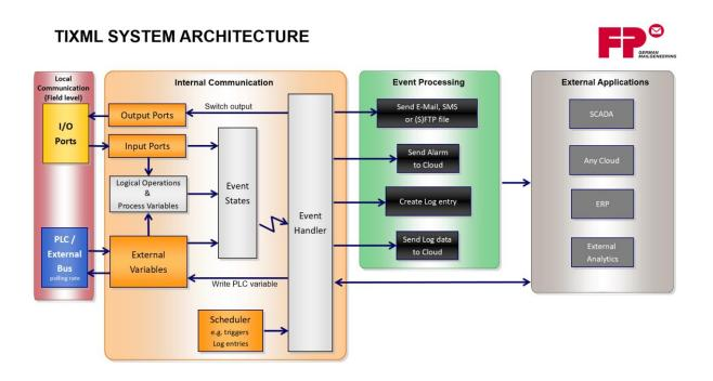
At first there is the field level "Local Communication" which may be a PLC connected via serial port or some switches and measurmenet instruments connected to the FP Gateway I/O ports. The configuration of PLCs is documented in a separate "PLC TiXML Manual".
