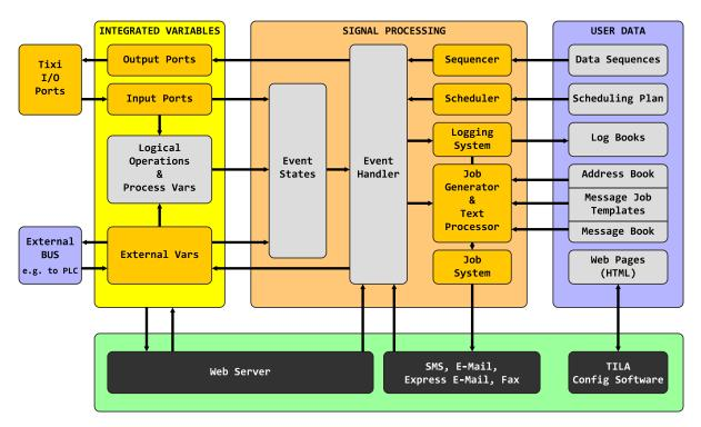
The process detects the changes of variables, e.g. the analog input which is mapped to the process variable path /Process/MB/A/AI/PO.
